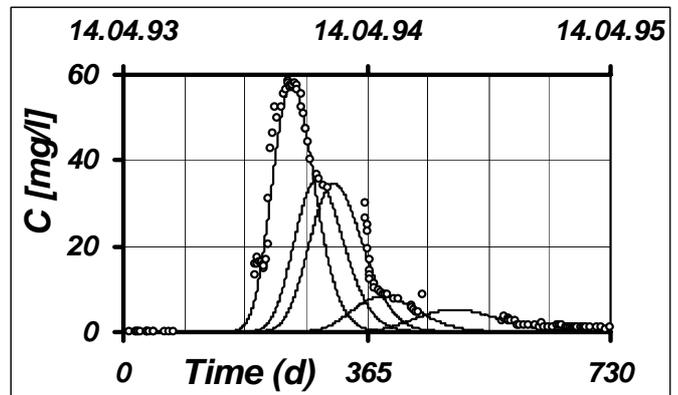
Figure 5. Numerical modelling of the tracer breakthrough curve (150 cm below surface) using the analytical solution of the transport equation.
