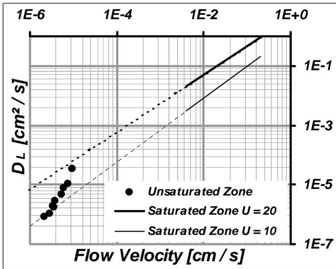
Figure 4. Dependency of the longitudinal dispersion coefficient ( $D_L$ ) from flow velocity in the unsaturated zone in comparison to saturated sand (Klotz & Moser 1974).
