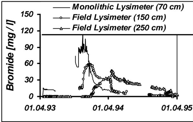
Figure 1. Comparison of bromide concentration breakthrough curves in different depths (70, 150 and 250 cm below surface).
