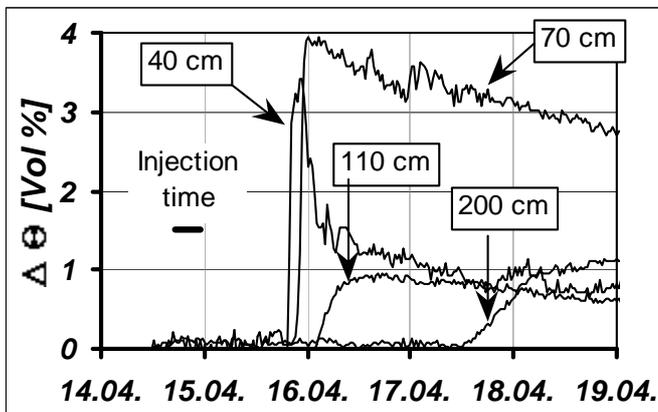
Figure 2. Changing of water content in different depth (40, 70, 110 and 200 cm below surface) as a hydraulic reaction on irrigation of 40 mm at injection time.
