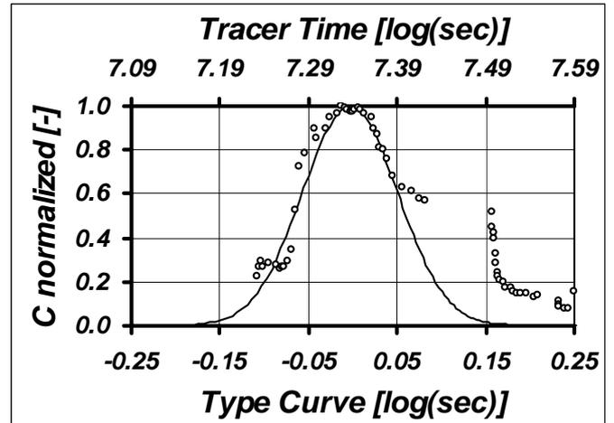
Figure 3. Fitting of Peclet Type Curve on the tracer breakthrough curve in 150 cm below surface.
