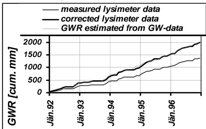
Figure 6. Comparison of cumulated sum of groundwater recharge (GWR [cum. mm]) between measured lysimeter data and corrected lysimeter data to ground water recharge estimated from ground water data (GW-data).
