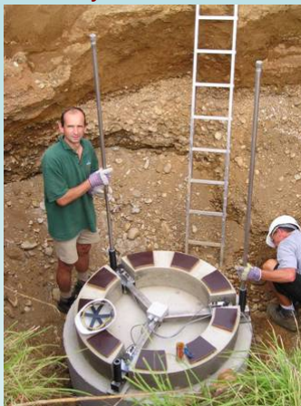
Weighing equipment (3 load cells) in Wagna picture: C. Lanthaler, August 2004
